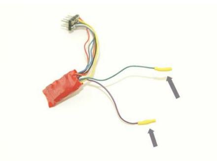
Figure 4. Covering the ends of the extra function wires
