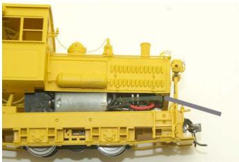
Figure 7. When removing the shell be careful not the hit the radiator and the circuit board
