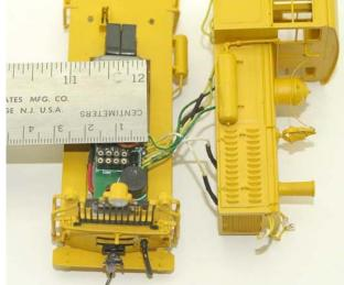
Figure 3. The overall width and socket position of an integrated socket decoder
