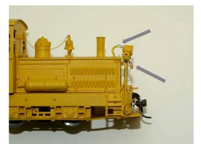
Figure 5. Removing the bulbs from the head light and front marker lights
