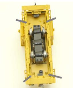
Figure 6. The screws that hold the shell to the frame
